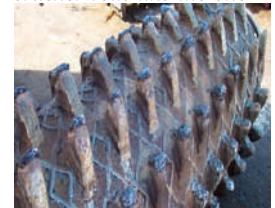
T170 is used to protect key wear points on crusher rolls like the one
