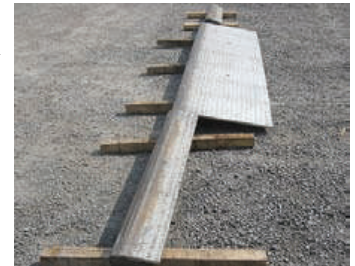
On the 'bullnose' or front lip of the screed, FCAW is used to apply TWP57.
