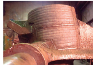
The coal-crushing trunion below is lined with T156.
