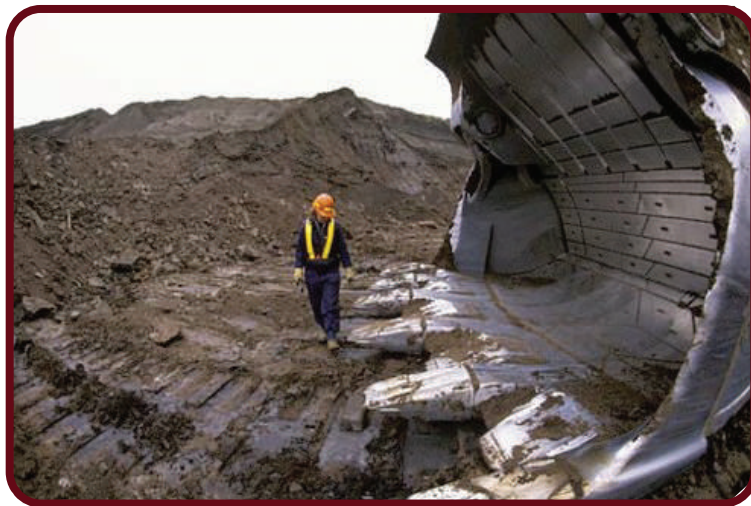
Trimay-lined shovel with Trimay bucket teeth
